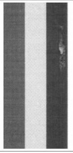
Although there were no visible signs of drum damage, the latter has caused the white marks that appeared at regular intervals along the right edge of output produced by Brand F's eighth cartridge.
