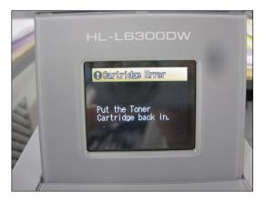
The first Brand K toner cartridge could not be recognized by the device, generating an error code upon installation.
